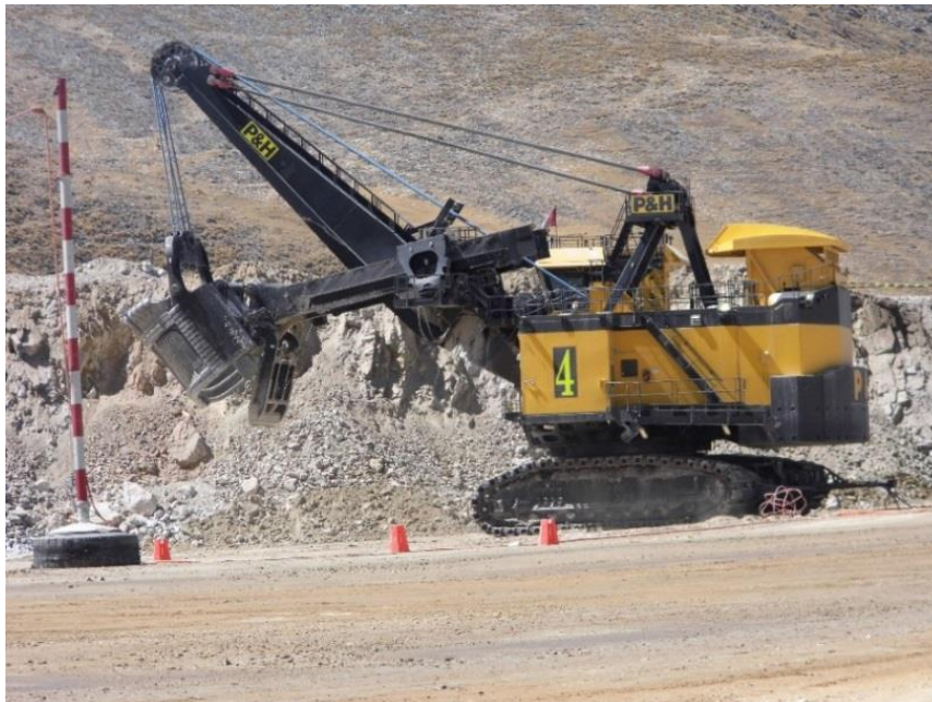
Figura 3.14: Pala Electrica #4 PyH 4100XPC
