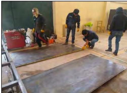
Figura 5.2: Plancha comercial ASTM A36
