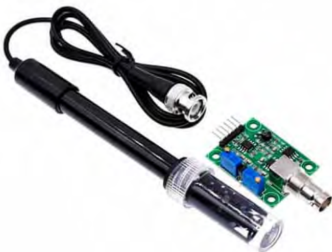
Figura 5 Sensor de PH-4502C
