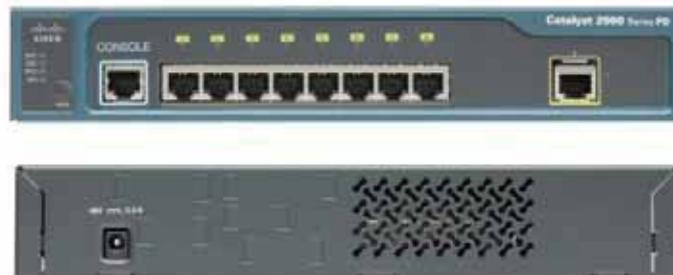
*Fig. 4.45: Switch cisco WS-C2960PD-8TT-L*
