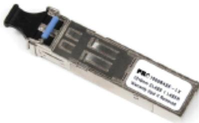
The GLC-LH-SMD is programmed to be fully compatible and functional with all intended Cisco Series switching devices. This SFP optical transceiver is based on the Gigabit Ethernet IEEE 802.3 standard and is designed to be compliant with SFF-8472 SFP Multi-source Agreement (MSA). This module is designed for single mode fiber and operates at a nominal wavelength of 1310nm.
