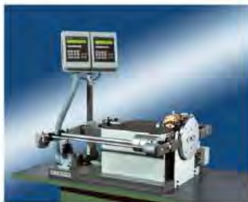
With multi-axis equipment, the axial and tangential moments can also be measured. This is especially necessary for wide chord, heavy blades. With the universal scale only the radial moment is determined.
