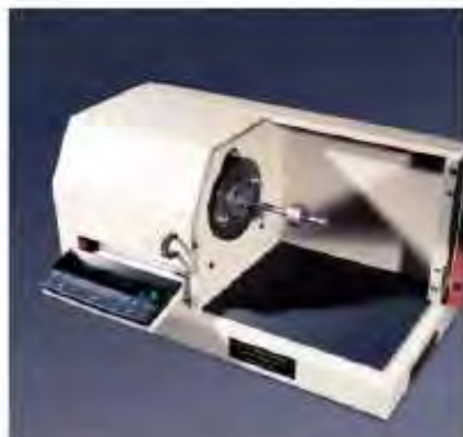
The central element of the Schenck Rotec moment weighing scale is a solid, horizontal beam mounted friction-free on knife-edges. With a blade mounted on the circular flange, the moment is determined by a precision balance and the lever-arm. In the case of universal scales, the important radial moment is determined. A digital readout device and display instrument ensures a broad measurement range along with high display sensitivity.
