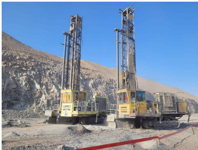
Figura 2: Perforadora DML, diametro de 9" taladros buffer.
